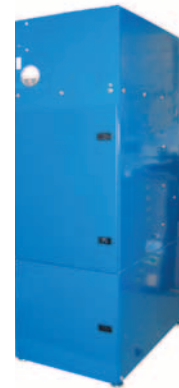
Diesel soot and ash removed by the cleaning process are captured in a servicable filter located in the lower portion of the cabinet.
